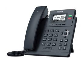
Yealink (SIP-T31P) 2 Line IP phone, 2.3" 132x64 pixel Graphical LCD, 2x Fast Ethernet Ports, 2 Program keys/BLF/XML/HDV
